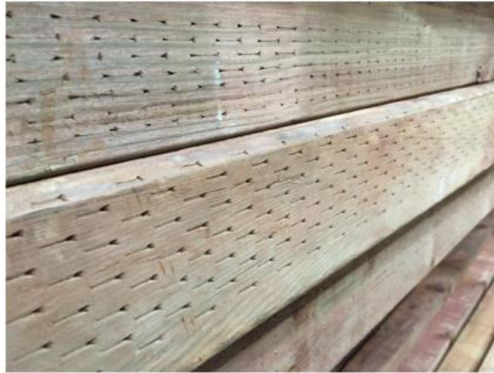
Photo 1. Pressure treated wood showing indentations
